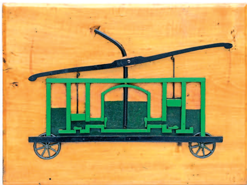
Fig. 12: Relief image – longitudinal section through an old fire pump; Technical Museum in Brno, Czech Republic; Photo: Eva Řezáčová
